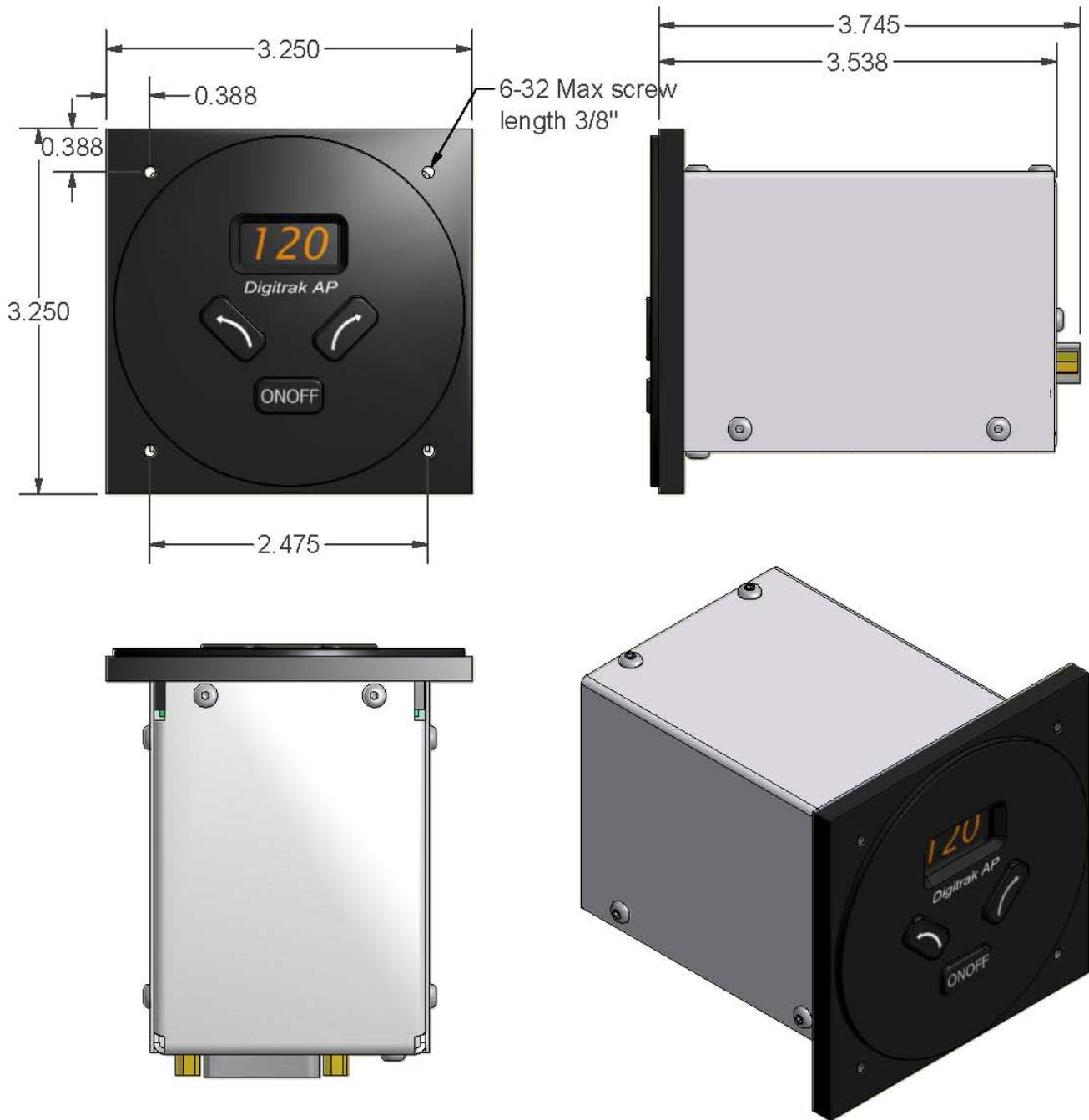
**MOUNTS IN STANDARD 3 1/8" INSTRUMENT HOLE**
